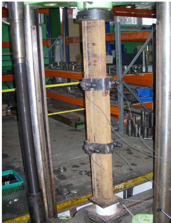
Fig. 1. The method of testing a friction joint at axial compression
