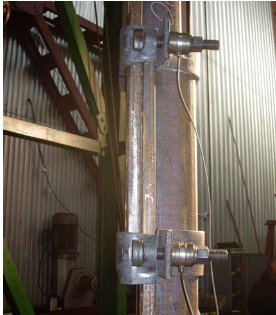
Fig. 2. Method of assembly of sleeve strain gauges for the measurement of values of axial forces in the bolts of stirrups
