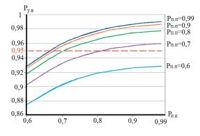
Fig. 2. Dependence of GSC effectiveness (  $P_{\rm S,f}$  ) on  $P_{\rm c,c}$  and  $P_{\rm c,r}$  during placement of four  $SS_{\rm S}$  in pairs in far and close control zones
