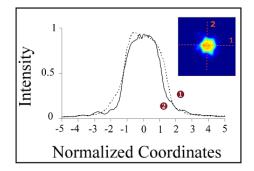
Fig. 9. Distribution of the output power with a hollow core PCF
