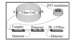
Fig. 1. Scheme of fiber optic gyroscope
