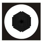
Fig. 6. An example of a photonic crystal fiber with a hollow core diameter of about 30 microns
