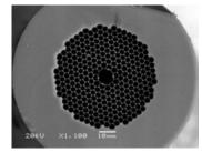
Fig. 4. Hollow core fiber cross section of core and cladding region
