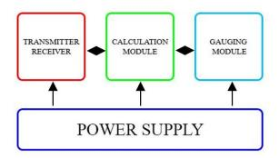
Fig. 3. A standard sensor node within a wireless network
