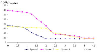
Fig. 1. Change of the concentration of ammonium nitrogen C ( $NH_4^+$ ) depending on the time of hydraulic water retention (t) for various co-substrates: 1 – paper waste, 2 – reed, 3 – hemp (systems are listed in accordance with Table 2)
