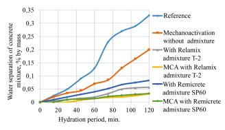
Fig. 4. Water separation of the concrete mixture
