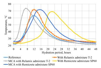
Fig. 1. Kinetics of the heat release of cement slurry
