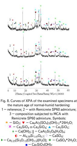
We see from the data of Tables 3, 4 that the MCA of cement suspension, along with the intensifiers of dispergation of Relamix T-2 and Remicrete SP60, leads to a deeper hydration of alite and belite, to the increase in the content of calcium hydrosilicates and ettringite in comparison to the compositions with the studied admixtures without MCA.
