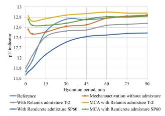
Fig. 2. Kinetics of pH of the liquid phase of cement slurry
