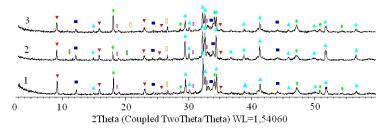
Fig. 5. Curves of XPA of the studied specimens at the age of 24 hours of normal-humid hardening: 1 – reference; 2 – with Relamix T-2 admixture; 3 – composition subjected to MCA with Relamix T-2 admixture. Symbols:  $[] - SiO_2; \lor - Ca_6Al_2(SO_4)_3(OH)_{12}*26H_2O; ]] - Ca_2SiO_4 \alpha - Ca_2SiO_4;$
