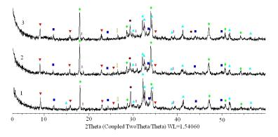
Fig. 6. Curves of XPA of the examined specimens at the mature age of normal-humid hardening: 1 - reference; 2 - with Relamix T-2 admixture; 3 - composition subjected to MCA with Relamix T-2 admixture. Symbols:  $-SiO_2$ ;  $-Ca_6Al_2(SO_4)_3(OH)_{12}*26H_2O$ ;  $-Ca_2SiO_4 \alpha$ -Ca<sub>2</sub>SiO<sub>4</sub>;  $-Ca_3SiO_5$ ;  $-Ca(OH)_2$ ;  $-Ca_2(AI, Fe^{+3})_2O_5$ ;  $-CaCO_3$
