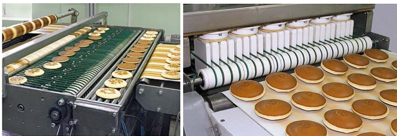
Fig. 6. Section of technological production line of confectionery products “PanCake” with cheese filling (industrial production at TOV PKG “Lisna Kazka”, Kharkiv)
