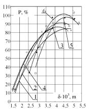
Fig. 9. Influence of the thickness of penetration through the surface layer of bulb on the degree of cleaning the bulbs at load factor 0.3 and shape and diameter of openings:
