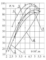
Fig. 11. Influence of the thickness of penetration through the surface layer of bulb on the degree of cleaning the bulbs at load factor 0.7 and shape and diameter of openings: 1 - circle, 12 mm; 2 - circle, 17 mm; 3 - circle, 22 mm; 4 - ellipse, 12×18 mm; 5 - ellipse, 17×23 mm; 6 - ellipse, 22×28 mm
