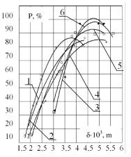
Fig. 10. Influence of the thickness of penetration through the surface layer of bulb on the degree of cleaning the bulbs at load factor 0.5 and shape and diameter of openings:
