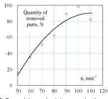
Fig. 12. Determining optimal drum rotation frequency by the indicator of quantity of removed parts of a bulb: × - experimental research; ------ - correlation curve
