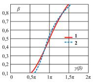
Fig. 5. Relationship between the coefficient of filling the drum and central angle of the segment with product: 1 - equation (9); 2 - approximate equation (26)
