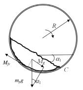
Fig. 4. Scheme of the forces that determine angle of lifting the layer of product a<sub>1</sub> under the first mode of the drum operation
