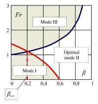
Fig. 6. Dependence of the Froude number's limiting values on the coefficient of filling the drum with onion
