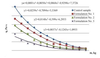
Fig. 5. Dependence of effective viscosity on the formulation composition of mince for cooked sausages
