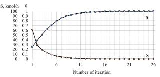
Fig. 1. Iterative calculation of static characteristics of normal operating mode of the rectifying column with the use of the classic  $\theta$ -method
