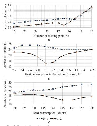
Fig. 5. Required number of iterations for calculating the rectifying column using the classic and modified  $\theta$ -methods: a – with different numbers of the feeding plate; b – with different thermal load of the boiler of the column bottom; c – with different feeding consumptions to the column
