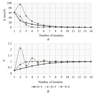
Fig. 4. Convergence of iterative calculations when using the classic (b=1) and modified  $\theta$ -methods: a – dependences of summary discrepancies of concentrations in the control section of the installation on the number of iteration; b – calculated values of coefficient  $\theta$
