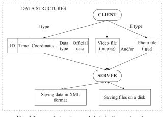
Fig. 3 Types of structures of data in the system for passenger traffic registration of public transport
