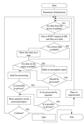
Fig. 4. Flowchart of working algorithm of the server
