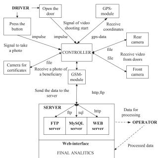
Fig. 2. Structure of data flow in the information model of the system for passenger traffic registration of public transport
