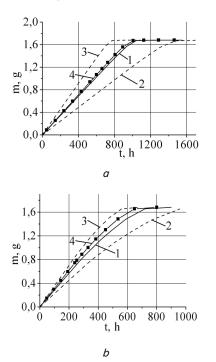
Fig. 4. Sedimentation curves, built in the coordinates of particle settling t and sediment mass m: a - suspension with the particles capable of forming a photonic crystal;
