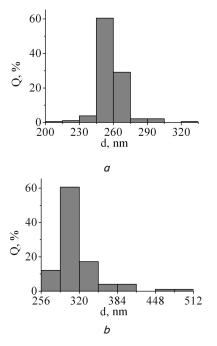
Fig. 3. Histogram of diameter distribution of synthesized particles d depending on the relative amount of particles in the interval of column of in histogram Q: *a* - particles, suitable for the formation of photonic crystal; *b* - particles that do not form photonic crystal
