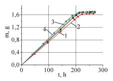
Fig. 5. Sedimentation curves of suspensions (dependence of sediment mass m on the settling time t) synthesized from tetraethoxysilane with different storage periods:
