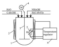
Fig. 1. Manufacturing section for the synthesis of SiO<sub>2</sub> particles by the hydrolysis of TEOS with different storage period: 1 - reactor; 2 - heating element; 3 - mixer; 4 - electric motor; 5 - thermistor; 6 - regulator
