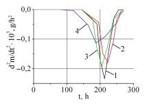
Fig. 6. Increase in the sediment mass in the sedimentation process of SiO<sub>2</sub> particles synthesized from TEOS with different storage periods: 1 - immediately after fractional distillation; 2 - in 48 hours after TEOS purification; 3 - in 96 hours after TEOS purification; 4 - in 144 hours
