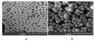
Fig. 2. Micrographs of the synthesized particles: *a* - suitable for the formation of photonic crystal; *b* - not forming photonic crystal
