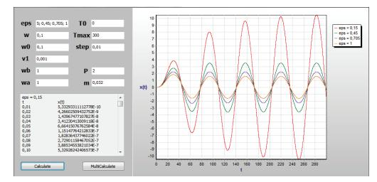
Fig. 8. Program interface for computer modeling of the work of gravimeter under the action of external disturbances
