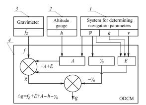
Fig. 1. Aviation gravimetric system for measuring anomalies in the acceleration of gravity
