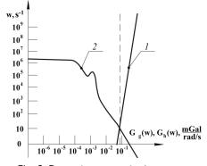
Fig. 2. Dependences on the frequency: 1 – AC vertical acceleration, 2 – spectral density of AG useful signal
