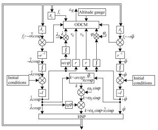
Fig. 6. Structural scheme of the system for determining the AG anomalies
