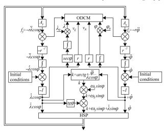
Fig. 5. Structural scheme of the system of AGS inertial navigation
