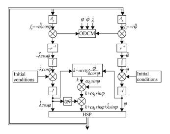
Fig. 4. Structural scheme of the AGS stabilization system
