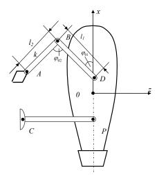
Fig. 1. Kinematic schematic of the manipulator on board and the element for fixing AUV
