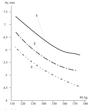
Fig. 7. Dependence of oscillation amplitude of vibratory separator on the oscillatory mass at the debalances angular velocity  $\omega_1 = \omega_2 = 110 \text{ s}^{-1}$ : 1 - suspension rigidity 10 kN/m; 2 - 13 kN/m; 3 - 16 kN/m
