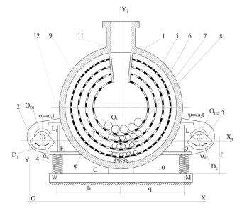
Fig. 2. Estimated scheme of the drum vibratory separator with concentric arrangement of sieves
