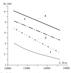
Fig. 8. Dependence of oscillation amplitude of vibratory separator on the magnitude of rigidity of the suspension springs: 1 – magnitude of the debalance radius
