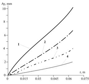
Fig. 6. Dependence of oscillation amplitude of vibratory separator on the radius of debalances:
