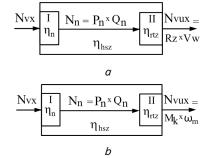
Fig. 6. Estimated models of HD with hydraulic engine:
