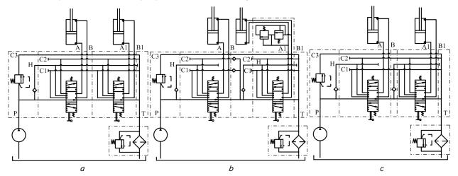
Fig. 4. Schemes of energy distribution from the pump to the hydraulic engines: a - parallel; b - sequential; c - individual. Designations in formulas (4) and (5) characterize the following: A, B, A1, B1 - cavities of hydraulic engines, the first and the second, respectively; C1, C2 - drain pipelines that are connected with the allocator;
