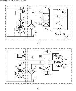
Fig. 5. Schematic of HD with two subsystems when using: a - hydraulic cylinder with the translationalmotion of rod; <math>b - hydraulic engine withthe rotational motion of shaft
