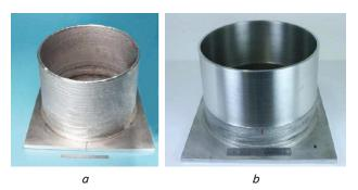
Fig. 5. Manufacturing of satellites cylindrical parts with variable wall thickness, made of aluminum alloys using arc welding (time of the part manufacturing -6 hours) [17]: a - after layer-by-layer building-up; <math>b - after machining
