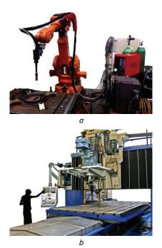
Fig. 10. Complexes for the implementation of welding additive technologies [9]: a - on the basis of anthropomorphic robot without machining; b - 3-axis complex with CNC-milling system
