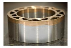
Fig. 7. Volumetric hollow part with internal stiffeners made of bimetal «structural steel – bronze Cu-3 % Si», obtained by means of arc welding (cladding) with current-carrying wire [17]
