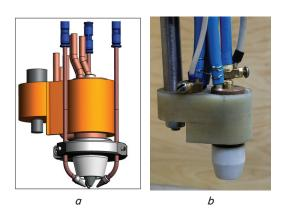
Fig. 16. Plazmatron for 3D printing of PLAZER 3D PW installation: a - computer 3D-model; b - external view
