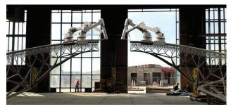
Fig. 13. The process of manufacturing a bridge using a welding 3D-printer [26]
