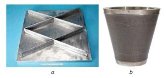
Fig. 3. Examples of three-dimensional products from carbon steel S355 [17]: *a* – panels with intersecting ribs without machining; *b* – part, machined after manufacturing
