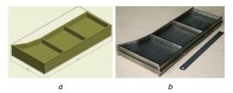
Fig. 8. Panels of complex shape with stiffeners made of Ti-6Al-4V alloy: *a* – volumetric model; *b* – panel, obtained by additive welding technology Wire-Arc Additive Manufacturing
