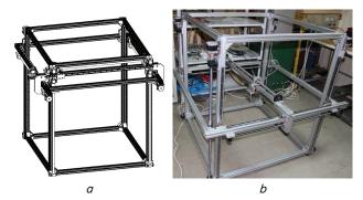
Fig. 15. Three-axis positioner of PLAZER 3D PW installation: a - computer 3D-model; b - external view
