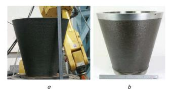
Fig. 4. Manufacturing of thin-walled conical parts of stainless steel [17]: a - before machining; b - duringmachining (the height of the parts is <math>- 1 m, the biggest diameter is 0.5 m)
