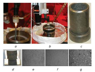
Fig. 12. Microplasma powder growing of volumetric products [11]: a – growing process; b – laboratory installation; c – hollow homogeneous cylinder (tool steel H-13); d – cross section of a hollow cylinder with a gradient composite structure (tool steel H13 + tungsten carbide); e – structure in the upper part of the cylinder; f – structure in the middle part; g – structure at the bottom
