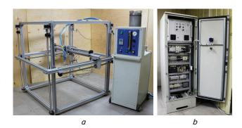
Fig. 17. The PLAZER 3D PW installation: a – manipulator with a plasmatron and a powder doser-feeder; b – view of power supply and control unit with the open front panel
