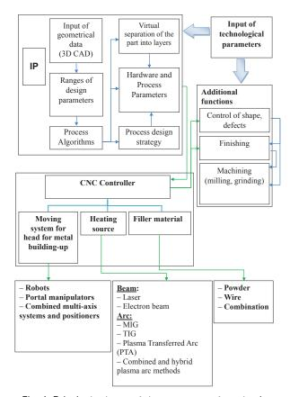
Fig. 1. Principal scheme of the processes of production of three-dimensional metal products using layer-by-layer additive building-up based on welding technologies
