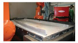
Fig. 9. Manufacturing of the aluminum structure of the aircraft wing [19]
