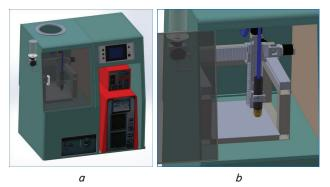
Fig. 14. Model of 3D-printer PLAZER 3D PW for the development of new plasma technologies for manufacturing volumetric products: *a* – general view; *b* – three-axis plasmatron positioner
