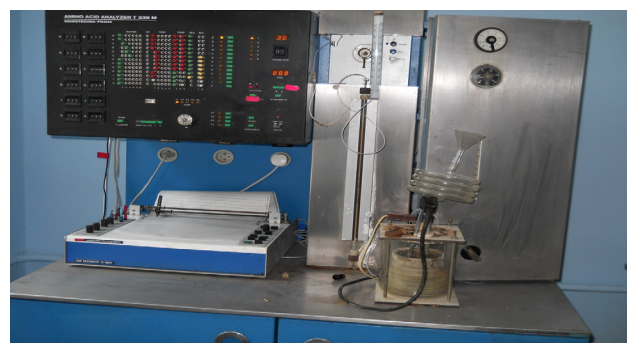
Fig. 5. The view of the device to determine the amino acid composition of the control and experimental batches of kefir
