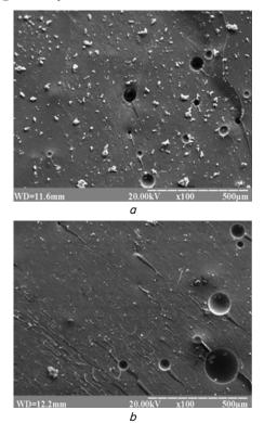
Fig. 9. Fractograms of the fracture of epoxy composites whose compositions are modified by ultrasound and filled with highly dispersed particles: a - iron of the type PZhR-3;  $b - \text{carbonyl iron} \times 100$
