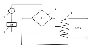
Fig. 2. Schematic of the installation for treating the composition in electromagnetic field: 1 – amperemeter; 2 – diode bridge; 3 – compensator; 4 –electromagnet
