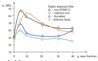
Fig. 7. Dependence of adhesive strength of the epoxy composites whose compositions are modified by ultrasound on the content and type of a highly dispersed filler
