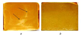
Fig. 8. General view of the surface of epoxy polymers: *a* – without pre-treatment; *b* – treating the composition with ultrasound
