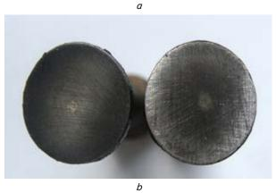
Fig. 6. General view of the surface of adhesive bond of the epoxy composite coatings, filled with highly dispersed zirconium powder, a – without treatment, b –treatment of the compositions in electromagnetic field
