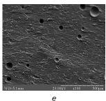
Fig. 4. Fractograms of the fracture of epoxy composites filled with highly dispersed particles: a - iron of the type PZh-3; b - carbonyl iron; c - ftoroplast (6 mass fractions); <math>d - ftoroplast (30 mass fractions); e - zirconium, ×100
