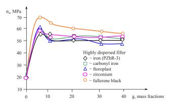
Fig. 5. Dependence of adhesive strength of the epoxy composites whose compositions are modified in the electromagnetic field on the content and type of a highly dispersed filler
