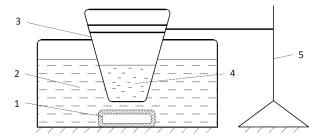
Fig. 1. Schematic of the installation for treating the composition with ultrasound: 1 - the source of radiation; 2 - medium (water); 3 - container; 4 - composition; 5 - tripod
