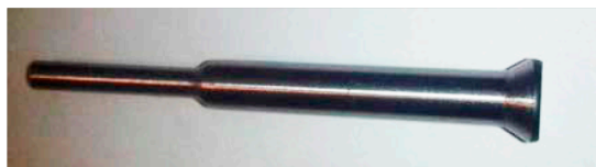
Fig. 2. General view of the punch made of steel 40KH
