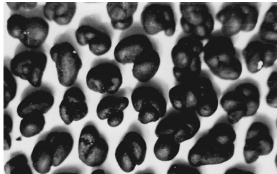
Fig. 8. Coal-oil fuel conglomerates of granules obtained based on Donetsk coal of 0–100 μm
