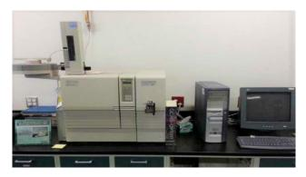
Fig. 2. Gas chromatograph GC-17A "Shimadzu" with the software "GC solution", (Japan)
