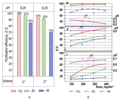
Fig. 5. Dependences of the efficiency of cleaning the washing waters of galvanic production: a — on the technological scheme and type of reagent-precipitant (column C' — using a calcined sediment; column C" — using a "fresh" sediment); b — on the dose of the precipitating reagent and pH of the solution at successive treatment of washing waters from the baths of zinc coating: I, III — magnetic structurizers; II — hydromechanical mixer
