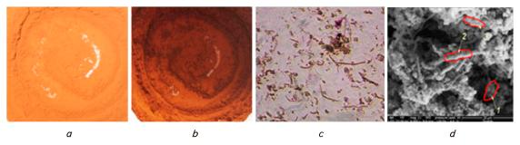
Fig. 3. Images of various types of the activated sediment: a - dried at t = 50 °C; b - dried at t = 600 °C; "fresh" sediment from matrices of iron bacteria: c - dried microscope ×400; d - dried matrices of iron bacteria: c - dried microscope ×400; d - dried matrices of iron bacteria: dried microscope ×400; d - dried matrices of iron bacteria: dried matrices of iron bacteria:
