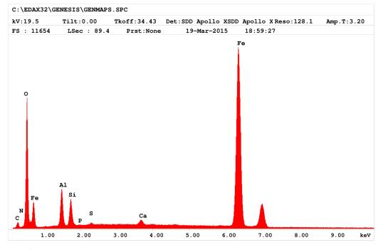
Fig. 6. X-ray spectral microanalysis of the sediment of the surface of the bacterium Leptothrix case
