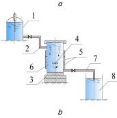
Fig. 1. Schematics of pilot installations for the removal of IHM: a – from technical groundwater: 1 – capacity of the source water; 2 – reactor tank; 3 – magnetic mixer; 4 – filter; 5 – capacity for filtrate collecting; 6 – Kamovsky pump; b – from flushing waters from galvanic production: 1 – a tank with the solution of flushing water; 2 – water supply to the column; 3, 4 – magnetic mixer; 5 – blocks of constant magnets; 6 – column structurizer; 7 – water drainage; 8 – mixer
