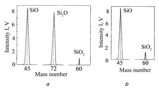
Fig. 3. A mass spectrogram of globular inclusions, isolated from steel E3 (Fig. 1): *a* – brownish-red; *b* – with a decay structure
