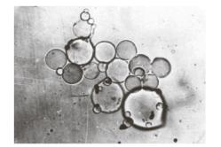
Fig. 1. Globular inclusions, isolated from steel E3. Light passing (×400)
