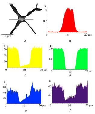
Fig. 8. Distribution of some chemical elements in graphite inclusions of gray cast iron: a - inclusion of graphite and a scanning line by a microprobe; b - distribution of carbon; c - distribution of silicon; d - distribution of iron; e - distribution of oxygen; f - distribution of sulfur
