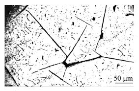
Fig. 6. Rosette and rectilinear-plate forms of graphite
