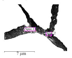
Fig. 9. Locations by the local micro-X-ray spectral analysis of graphite inclusions
