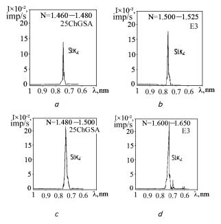
Fig. 2. Spectra of characteristic radiation of globular inclusions, isolated from steels 25ChGSA and E3:
