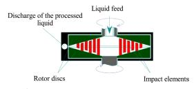
Fig. 1. Schematic diagram of the hydrocavitation device
