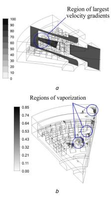
Fig. 8. Distribution of flow rates and the region of vaporization in the fuel-flow section of the rotary cavitation device: a - distribution of flow velocities in the fuel-flow section; b - regions of vaporization in the fuel-flow section
