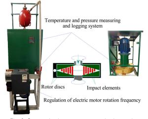
Fig. 9. Schematic view of a rotary cavitation device
