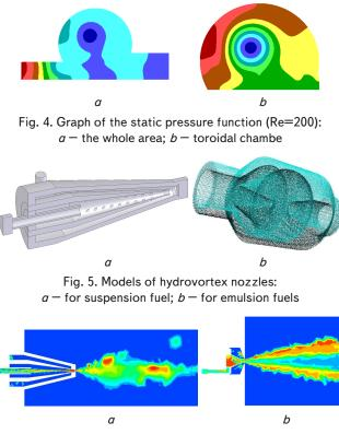
Fig. 6. Results of computer modeling of the torch at the nozzle outlet: a - for suspension fuels; b - for emulsion fuels
