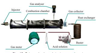
Fig. 10. Schematic view of the burner unit and the flue gas sampling system
