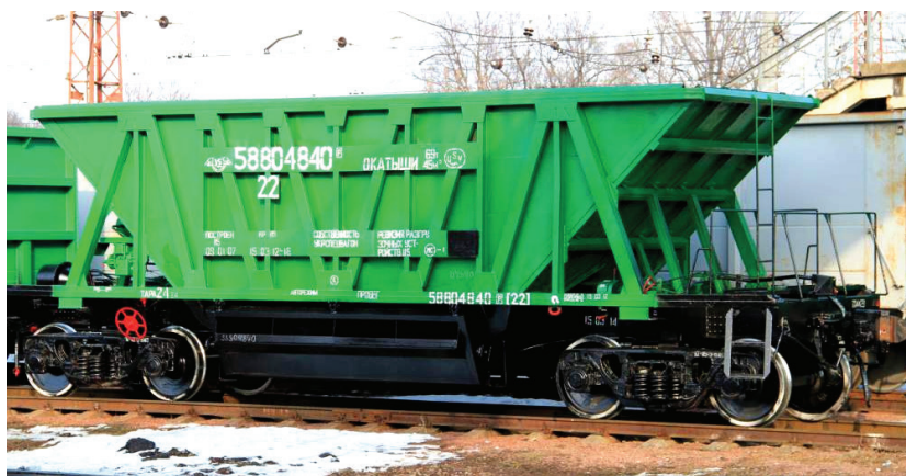
Fig. 6. Wagon for transporting iron ore pellets and agglomerate, model 20-9749
