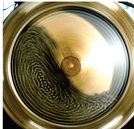
Fig. 6. The fill's flow patterns at \psi_\omega=0.75 , \kappa=0.35 , d/(2R)=0.026 and smooth chamber surface: a – calculated; b – experimental
