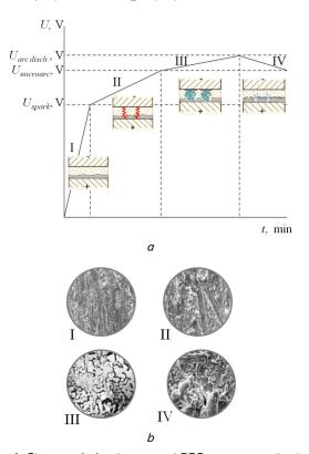
Fig. 1. Characteristic of stages of PEO-treatment of valve metals: *a* − chronograms of inter-electrode voltage, *b* − surface morphology of the system Al | Al<sub>2</sub>O<sub>3</sub>·CoO<sub>x</sub> at different stages of PEO. Magnification ×1000
