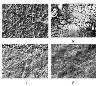
Fig. 4. Impact of current density on surface morphology of the oxide-metallic catalytic systems on AK12M2MgN:  $a - AI \mid AI_2O_3 \cdot CoO_y \cdot 5 A/dm^2$ ,  $b - AI \mid AI_2O_3 \cdot CoO_y \cdot 10 A/dm^2$ ,  $c - AI \mid AI_2O_3 \cdot MnO_v \cdot 15 A/dm^2$ ,  $d - AI \mid AI_2O_3 \cdot MnO_v \cdot 20 A/dm^2$
