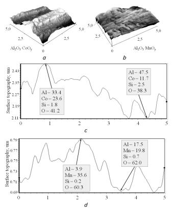
Fig. 5. 3D maps and cross-section profiles of the oxide-metallic systems: a, c – Al | Al<sub>2</sub>O<sub>3</sub>·CoO<sub>y</sub>, b, d – Al | Al<sub>2</sub>O<sub>3</sub>·MnO<sub>y</sub>. Scanning area is  $5\times5$   $\mu$ m
