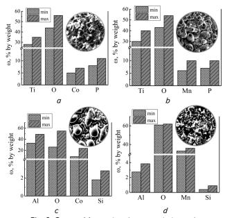
Fig. 3. Composition and surface morphology of the oxide-metallic catalytic systems:  $a - \text{Ti} \mid \text{TiO}_2 \cdot \text{CoO}_y$ ,  $b - \text{Ti} \mid \text{TiO}_2 \cdot \text{MnO}_y$ ,  $c - \text{Al} \mid \text{Al}_2\text{O}_3 \cdot \text{CoO}_y$ ,  $d - \text{Al} \mid \text{Al}_2\text{O}_3 \cdot \text{MnO}_y$ . Magnification  $\times 500$
