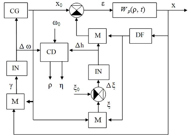
Fig. 3. Block diagram of the intermediate measuring transducer: CG – controlled generator; IN – integrator; M – multiplier; DF – differentiation unit; CD – computing device;  $x, \epsilon$  – system coordinates;  $\rho, \eta$  – controlled density and viscosity;  $p$  – differentiation operator;  $x_0 = a_0 \sin(\omega_0 + \Delta\omega) -$  input signal;  $\gamma, \xi$  – control coordinates of the adaptation circuits;  $W_p(p, t)$  – resonator transmission function;  $t$  – time coordinate
