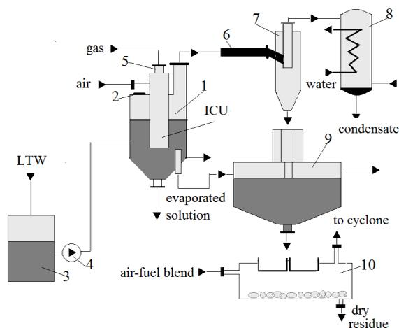
Fig. 1. LTW thermal treatment plant based on the ICU:
