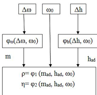
Fig. 4. Block diagram for density and viscosity calculation in multi-circuit control of parameters
