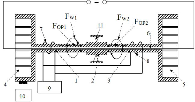
Fig. 2. Resonator of the immersed measuring transducer of liquid density and viscosity: 1 – elastic non-magnetic connector; 2, 3 – magnetoelastic rods; 4, 5 – cylinders with partitions; 6 – winding of the DC voltage passing through an internal cavity of both rods; 7, 8 – coaxial windings; 9 – controlled generator; 10 – receiver of torsional vibrations; 11 – resonator fixing column
