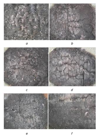
Fig. 2. Results of charring depth of a wooden construction: *a* – untreated; treated with: *b* – organic coating with the addition of aluminosilicate microspheres, *c* – organic coating with the addition of perlite, *d* – organic coating with the addition of basaltic scales, *e* – organic coating with the addition of sludge, *f* – organic coating with the addition of ashes
