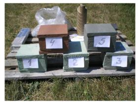
Fig. 1. Model samples of containers for the storage of weapons and ammunition that were treated with an organic coating with an addition of: 1 – aluminosilicate microspheres; 2 – perlite; 3 – basalt scales; 4 – metallurgical sludge; 5 – ashes
