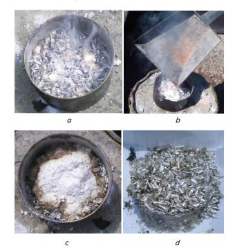
Fig. 4. Results of tests of extinguishing magnesium flame with a model sample of dry mixtures coating with the addition of minerals: a – magnesium ignition, b – extinguishing of flame, c – formation of combustible substance of the insulation layer on a surface, d – results of extinguishing
