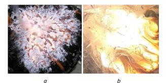
Fig. 3. Results of extinguishing magnesium flame with wet sand: a - combustion of magnesium; b - throwing of a wet sand in a magnesium flame
