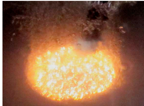
Fig. 1. The type of microdischarges in microarc oxidation of aluminum surface
