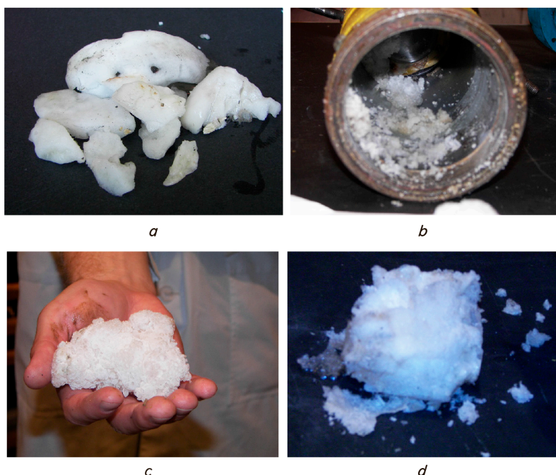
Fig. 6. Gas hydrates obtained in the experimental studies under laboratory conditions: a – condensed gas hydrate; b – gas hydrate crystals in the reactor of a laboratory installation; c, d – loose gas hydrate
