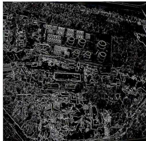
Fig. 6. Result of segmentation of the original image (Fig. 5) by the evolutionary method
