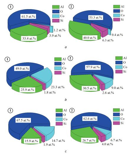
Fig. 5. Chemical composition of plots 1 and 2 (Fig. 4) on oxide coatings obtained in electrolytes of following composition, mol/dm<sup>3</sup>:  $a - 0.4 \text{ K}_4\text{P}_2\text{O}_7$ , 0.05 CoSO<sub>4</sub>;  $b - 0.4 \text{ K}_4\text{P}_2\text{O}_7$ , 0.1 CoSO<sub>4</sub>;  $c - 0.6 \text{ K}_4\text{P}_2\text{O}_7$ , 0.2 CoSO<sub>4</sub>
