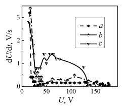
Fig. 2. Rate of voltage change during PEO of AK12M2MgN in electrolytes with different composition, mol/dm<sup>3</sup>:  $a - 0.4 \text{ K}_4\text{P}_2\text{O}_7$ , 0.05 CoSO<sub>4</sub>;  $b - 0.4 \text{ K}_4\text{P}_2\text{O}_7$ , 0.1 CoSO<sub>4</sub>;  $c - 0.6 \text{ K}_4\text{P}_2\text{O}_7$ , 0.2 CoSO<sub>4</sub>
