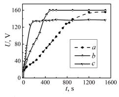
Fig. 1. Chronograms of forming voltage during PEO of AK12M2MgN in electrolytes of the following composition, mol/dm<sup>3</sup>:  $a - 0.4 \text{ K}_4\text{P}_2\text{O}_7, 0.05 \text{ CoSO}_4; b - 0.4 \text{ K}_4\text{P}_2\text{O}_7, 0.1 \text{ CoSO}_4;$  $c - 0.6 \text{ K}_4\text{P}_2\text{O}_7, 0.2 \text{ CoSO}_4$
