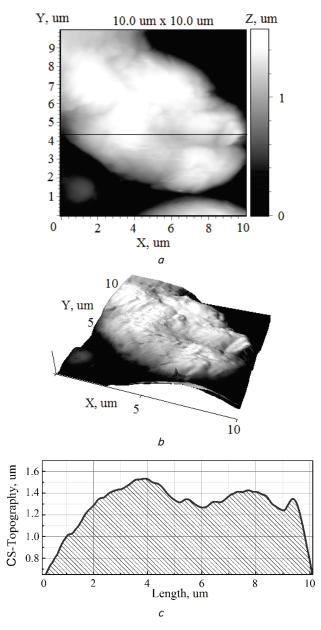
Fig. 6. Surface of the cobalt-containing oxide PEO-coating on AK12M2MgN obtained from electrolyte 0.4 mol/dm<sup>3</sup>  $K_4P_2O_7$ , 0.1 mol/dm<sup>3</sup> CoSO<sub>4</sub>: a - 2D-map, b - 3D-map, c - cross-section profile. Scanning area 10×10 µm
