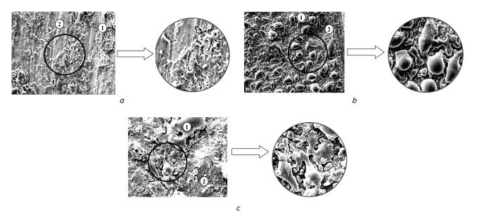
Fig. 4. Surface morphology of oxide coatings on AK12M2MgN, formed on electrolytes of following composition, mol/dm<sup>3</sup>:  $a - 0.4 \text{ K}_4\text{P}_2\text{O}_7$ , 0.05 CoSO<sub>4</sub>;  $b - 0.4 \text{ K}_4\text{P}_2\text{O}_7$ , 0.1 CoSO<sub>4</sub>;  $c - 0.6 \text{ K}_4\text{P}_2\text{O}_7$ , 0.2 CoSO<sub>4</sub>. Magnification ×500 and 1000
