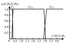
Fig. 3. Membership function of term sets of the input linguistic variable  $C_2H_2/C_2H_4$  after training
