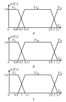
Fig. 2. Membership functions:  $a - input variable of C_2H_2/C_2H_4; b - input variable of CH_4/H_2;$  $c - input variable of C_2H_4/C_2H_6$
