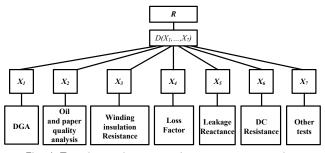
Fig. 1. The hierarchical block diagram for the technical condition assessment of power transformers
