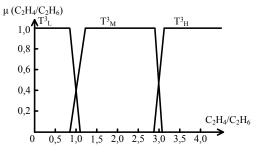
Fig. 5. Membership function of term-sets of the input linguistic variable  $C_2H_4/C_2H_6$  after training
