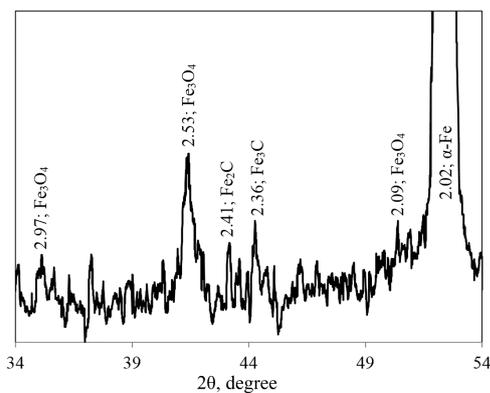
Fig. 4. A fragment of a diffractogram of metallization products with a degree of extraction of 97 % with a content of 50 mass % of 12Cr18Ni10Ti steel scale in the charge as to Fig. 1
