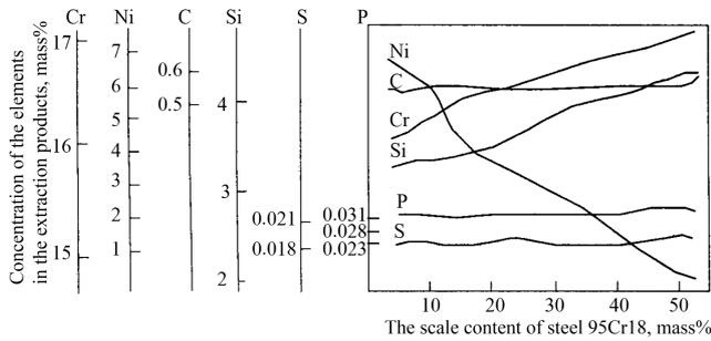
Fig. 2. Dependence of the chemical structure of the extraction products on the content of 95Cr18 steel scale in the charge
