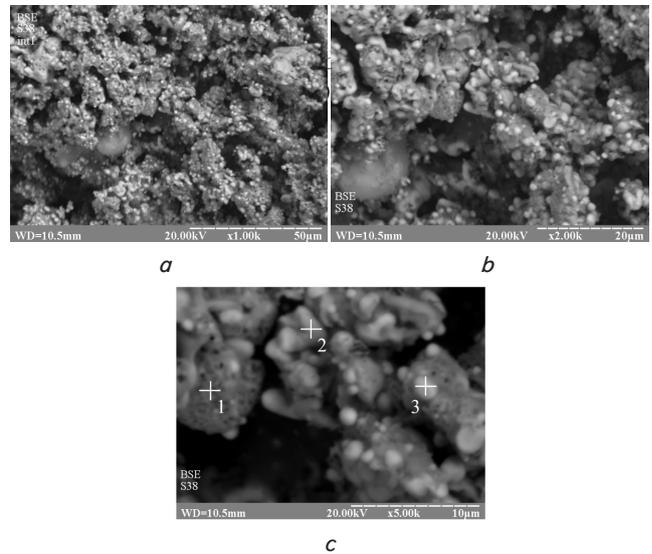
Fig. 5. The microstructure of the metallization products with an extraction degree of 97 % with a content of 50 mass % of 12Cr18Ni10Ti steel scale in the charge as to Fig. 1, zoomed in as follows: a –  $\times 1000$ , b –  $\times 2000$ , and c –  $\times 5000$
