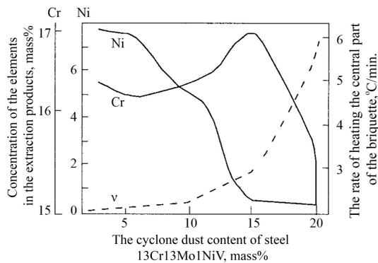
Fig. 3. Dependence of the chemical structure of the extraction products and the increase of the heating rate of the central part of the briquette on the content of 13Cr13Mo1NiV steel cyclone dust in the charge
