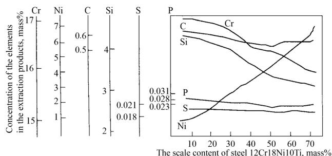
Fig. 1. Dependence of the chemical structure of the extraction products on the content of 12Cr18Ni10Ti steel scale in the charge
