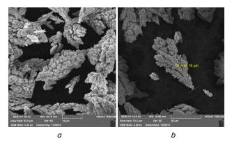
Fig. 4 SEM images of nickel powder prepared with Trilon B additive. Magnification:  $a - \times 1,330$ ,  $b - \times 4,000$
