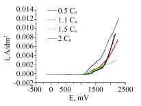
Fig. 1. Anodic polarization curves of the nickel electrode in electrolytes for nickel powder synthesis with different ammonia concentrations
