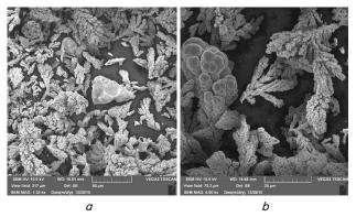
Fig. 3. SEM images of nickel powder prepared without Trilon B additive. Magnification:  $a - \times 1,330$ ,  $b - \times 4,000$
