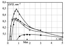
Fig. 2. Differential function of distribution of pores by radii in multicomponent natural puree according to formulation ratio:  $\bigcirc -(1a) 60 \%$  of apple, 30 % of cranberry, 10 % of hawthorn;  $\triangle -(1b) - 65 \%$  of apple, 25 % of cranberry, 10 % of hawthorn;  $\bigcirc -(1c) - 55 \%$  of apple, 40 % of cranberry, 5 % of hawthorn;  $\blacksquare -$  control (100 % of apple raw material)
