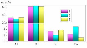
Fig. 3. Composition of  $AI_2O_3$ ·CoO<sub>x</sub> coatings (Fig. 2), formed at different current densities,  $A/dm^2$ : 1 - 3; 2 - 5; 3 - 10
