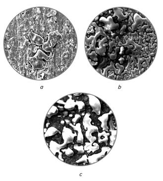
Fig. 2. Surface morphology of  $Al_2O_3 \cdot CoO_x$  coatings, obtained at different current densities,  $A/dm^2$ : a - 3; b - 5; c - 10. Magnification ×500
