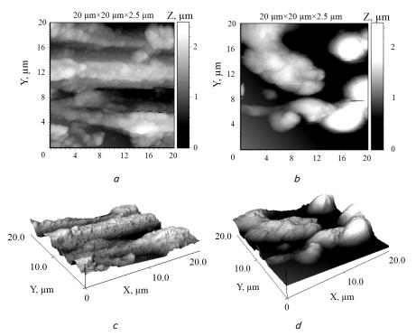
Fig. 6. Topography of the surface of  $Al_2O_3 \cdot CoO_x$  coating on AL25, formed at current density of 5 A/dm<sup>2</sup> within, min: *a*, *c*- 10, *b*, *d*- 20, *a*, *b* - 2D-map, *c*, *d* - 3D-map. Scan area  $20 \times 20 \ \mu m$
