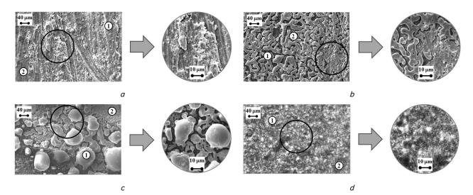
Fig. 4. Morphology of surface of Al<sub>2</sub>O<sub>3</sub>·CoO<sub>x</sub> coating on AL25, obtained in diphosphate electrolyte at different oxidation time, min: a - 10; b - 20; c - 40; d - 60. Magnification ×500 and 1,000
