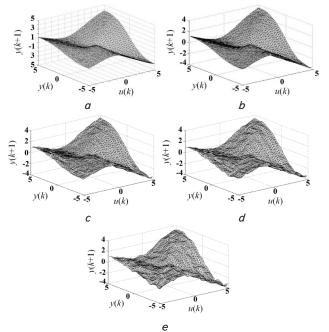
Fig. 7. Results of experiment 5: a – surface described by equation (34); b – surface restored without hashing the information; c – results of the identification using hashing at m=500; d – at m=400; e – at m=350
