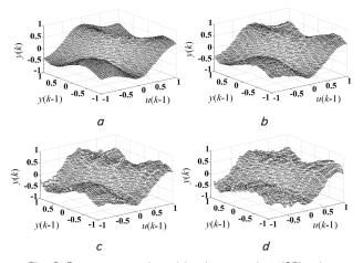
Fig. 2. Results of the identification of object (37) using rectangular membership functions: a – surface restored without the use of hashing; b – results of the identification using hashing at m=500; c – at m=400; d – at m=350
