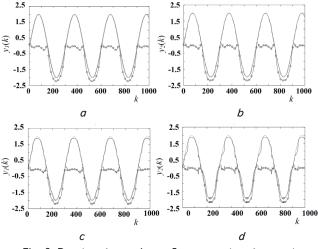
Fig. 8. Results of experiment 5: a - results of controls without using the hashing; b - using the hashing at m=500; c - at m=400; d - at m=350
