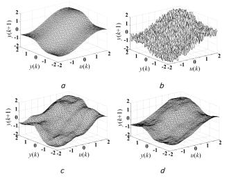
Fig. 4. Results of the identification of a very noisy object (38): a - reference surface; b - noisy surface; c - results of the identification using algorithm (27) with  $\gamma(k)=1$ ; d - with  $\gamma(k)$  modified in accordance with formula (28)
