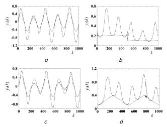
Fig. 6. Results of the work of a neural controller: a - for the first channel for a sinusoidal reference signal; b - for the second channel for a sinusoidal reference signal; c - for the first channel for a saw-shaped reference signal; d - for the second channel for a saw-shaped reference signal
