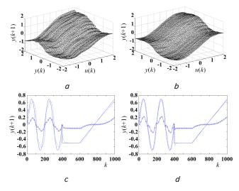
Fig. 5. Results of the identification and indirect control, without a reference model, of a very noisy object (38): a - results of the identification using algorithm (27) with  $\gamma(k)=1$ ; b - with parameter  $\gamma(k)$  that changes in line with (28); c, d - results of control
