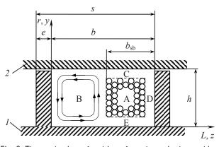
Fig. 3. The mechanism of melting of a polymer in the working channel of a single-screw extruder: 1 – a screw;
