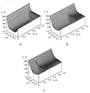
Fig. 5. Temperature fields in the screw channel at different values of the dimensionless coordinate L/D:
