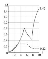
Fig. 3. Consumptions of compressed air in actuation of the PA with the base scheme No. 1 (solid line) and the energy-saving scheme No. 2 (dotted line)
