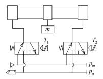
Fig. 1. Basic (elementary) scheme of the pneumatic actuator (scheme No. 1): *m* is mass of moving parts of the PA;  $p_m$  is pressure in the feed line of the PA;  $p_a$  is atmospheric pressure;  $T_1$ ,  $T_2$  are Boolean variables determining the states of the control electromagnets (T=1 for current on, T=0 for current off)
