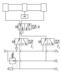
Fig. 2. Energy-saving scheme of the pneumatic actuator (scheme No. 2)
