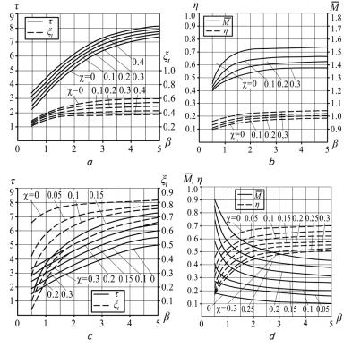
Fig. 5. Dependence of the main operational characteristics of the PA on the criteria of dynamic similarity  $\beta$  and  $\chi$ : scheme No. 1 (*a*, *b*); scheme No. 2 (*c*, *d*)
