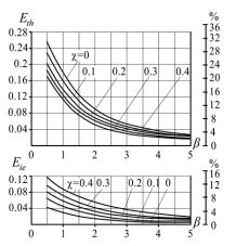
Fig. 6. Dependence of the loss of working capacity of compressed air for throttling ( $E_{th}$ ) and because of incompleteness of air expansion in the working chamber ( $E_{ie}$ ) on the  $\beta$  and  $\gamma$  criteria
