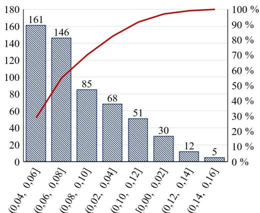
Fig. 2. Histogram of pores distribution according to dimensions of sample no. 5, plotted in program Origin based of the data, obtained with the help of ImageJ
