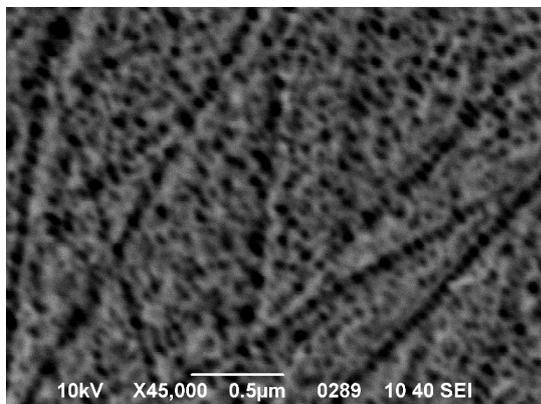
Fig. 1. REM-image of morphology of por-InP (sample No. 5)
