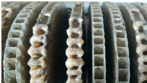
Fig. 2. Bioreactor disks with immobilized biomass
