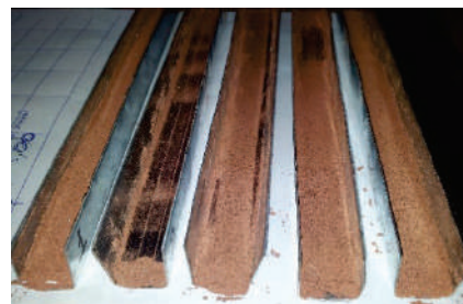
Fig. 11. Samples of the rolled powdered material in a metal sheath
