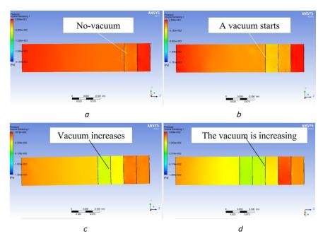
Fig. 11. Distribution of exhaust gas pressure in the filter-not-cut variation: a - Filters 2; b - Filters 3; c - Filters 4 and; d - Filters 5
