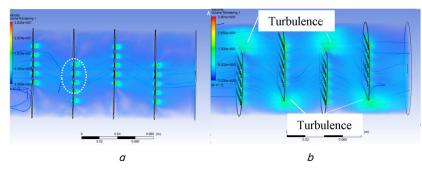
Fig. 9. The exhaust gas flow pattern passes through four Catalytic converters: a - Filter-not-cut and; b - Filter cut
