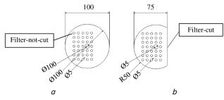
Fig. 1. Cut-filter model: *a* – Filter dimensions; *b* – Filter-not-cut model
