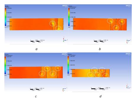
Fig. 12. Distribution of exhaust gas pressure on filter-cut variations: a - Filters 2; b - Filters 3; c - Filters 4 and; d - Filters 5
