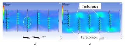
Fig. 10. The flue gas flow pattern passes through five Catalytic converters: a - Filter-not-cut and; b - Filter cut
