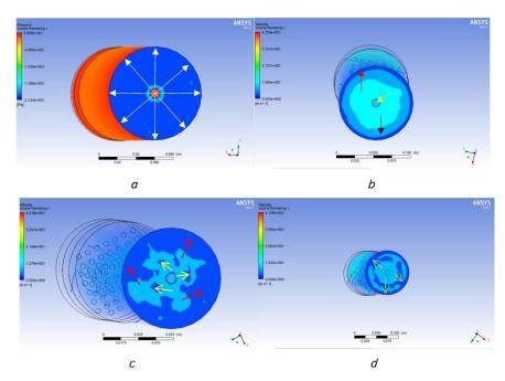
Fig. 13. Distribution of pressure on: a - Filter-not-cut 2; b - Filter-cut 2; c - Filter-not-cut 3 and; d - Filter cut 3
