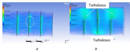
Fig. 8. The pattern of exhaust gas passes through three catalytic converters: a - Filter-not-cut and; b - Filter-cut
