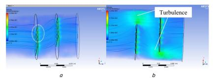
Fig. 7. The flue gas flow pattern passes through two Catalytic converters: a - Filter-not-cut and; b - Filter-cut
