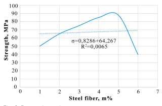
Fig. 6. Plot of fiber-reinforced concrete strength versus steel fiber content
