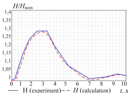
Fig. 2. Dependence of relative head of turbine on time
