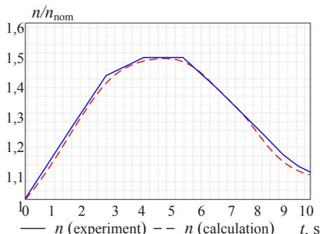
Fig. 1. Dependence of relative rotation frequency of turbine on time
