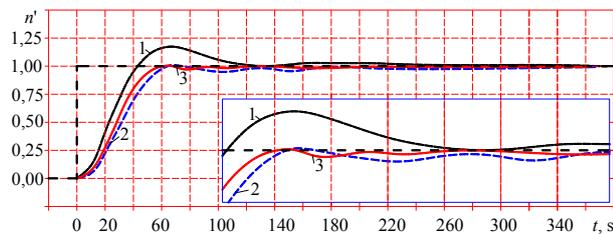
Fig. 4. Change in the relative frequency of rotation of a hydrogenerator unit when setting the load using different control algorithms: 1 – classic PID controller; 2 – proposed controller; 3 – controller with the technology Feed-forward with a reference model
