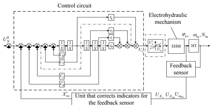
Fig. 5. Principal diagram of the astatic controller based on the solution to the inverse problem of dynamics
