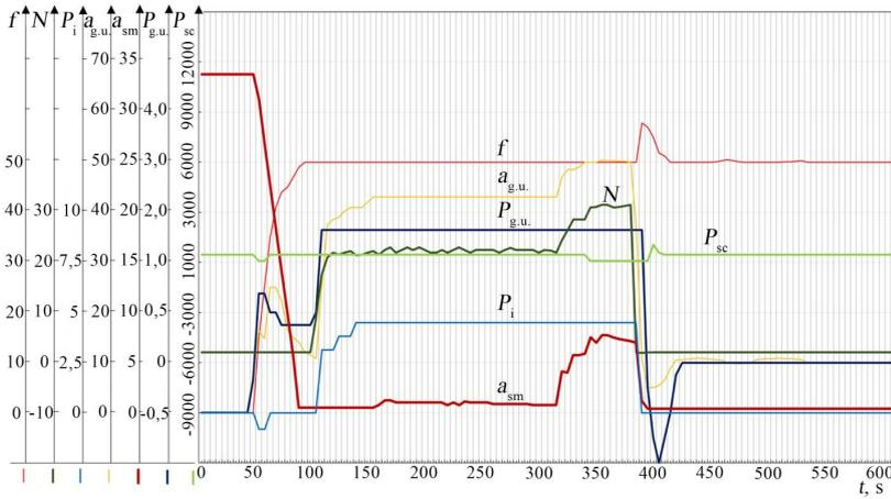
Fig. 3. Transient processes when changing a load at the hydrogenerator unit:  $f$  – current frequency, Hz;  $N$  – active capacity of the unit, MW;  $P_i$  – pressure before the impeller, kg/cm<sup>2</sup>;  $a_{g.u.}$  – position of the servomotor of the guiding unit, %;  $a_{sm}$  – position of the impeller’s servo motor, %;  $P_{g.u.}$  – pressure after the guiding unit, kg/cm<sup>2</sup>;  $P_{sc}$  – pressure in a spiral chamber, kg/cm<sup>2</sup>
