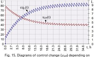
the level of resources  $(cq_L)$  in the buffering mechanism
