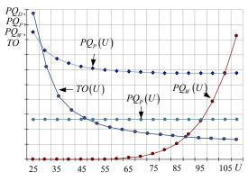
Fig. 4. Dependence of parameters of a process operation on control: control (U); power consumption ( $PQ_P$ ); a product of direct effect ( $PQ_D$ ); wear ( $PQ_W$ ); time of the process operation (PO)
